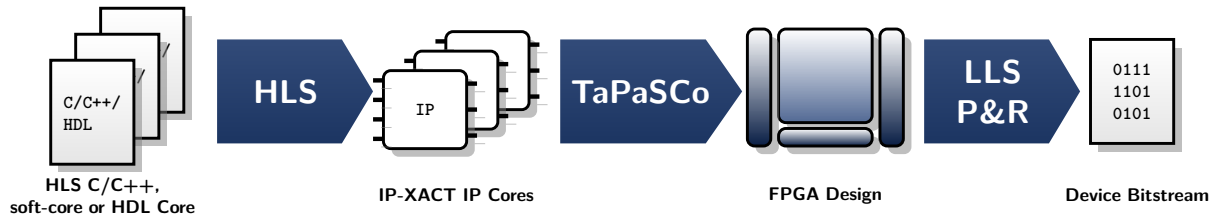
Fig. 2. TaPaSCo tool-flow, starting from the accelerator definition given as HDL-code, softcore IP, or C/C++-based HLS code. If necessary, HLS is automatically performed. After the user-specified composition of the architecture, a complete FPGA design for the requested target platform is automatically constructed, which will then be synthesized to a complete bitstream using the vendor's tool, e.g., Xilinx Vivado.
