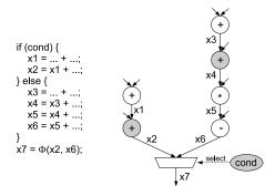
Fig. 1. Speculative data paths of different length. Gray highlighted operations denote currently available results.
