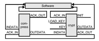
Fig. 1. Hardware pipeline used by software
